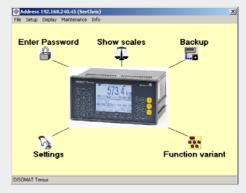
All parameter and calibration data are stored in the terminal to protect them from power failure. The real-time clock continues to run for at last seven days.
